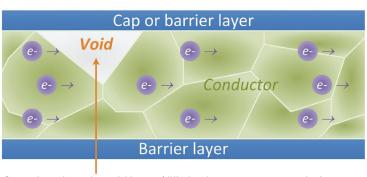
Copper has migrated out of this area (diffusion due to momentum transfer from traveling electrons). Voids typically locate at the cap interface, grain boundaries, and via bottoms and continue to grow under stress. After void formation, current must flow around the voids.
